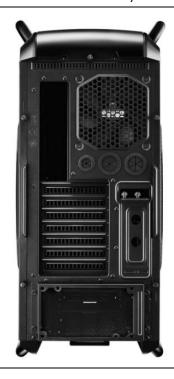
Rear (with liquid cooling tubing holes)
