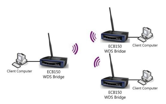
**Note**: WDS Bridge Mode does not act as an Access Point. Access Points linked by WDS are using the same frequency channel. More Access Points connected together may lower throughput. Please be aware to avoid loops in your wireless connection, otherwise enable Spanning Tree Function.
