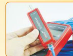
Verify Lan Cable Condition
