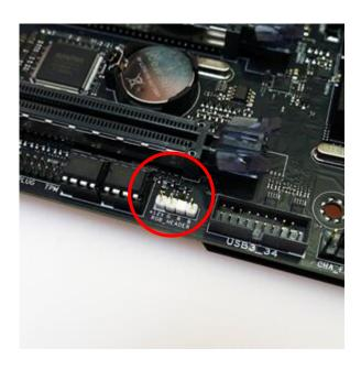
• 1) Require motherboard with Addressable RGB header to enable RGB lighting.
