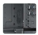
Cable grommets for better cable routing
