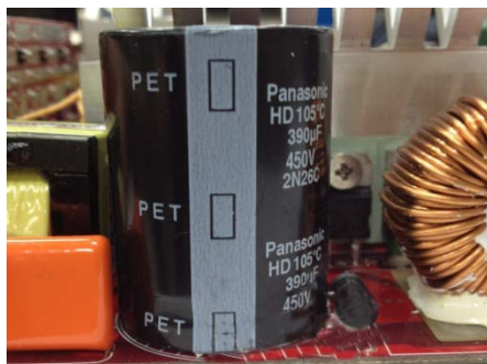
Japanese capacitor ensures an extended lifetime and excellent hold up times
