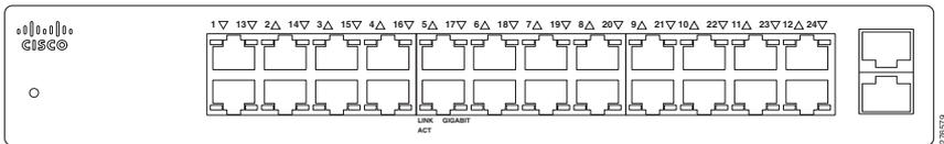
**RJ-45 Ethernet Ports**—Use these ports to connect network devices, such as computers, printers, and access points, to the switch. The auto-sensing, Ethernet (802.3) ports are used for wired network communications. Each Ethernet port supports network speeds of 10 Mbps, 100 Mbps, or 1000 Mbps.
